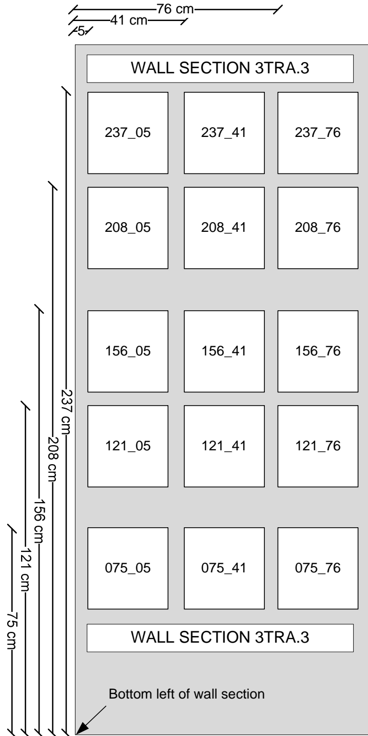
Figure 15 – Example of non-vertically aligned patch panel identification
